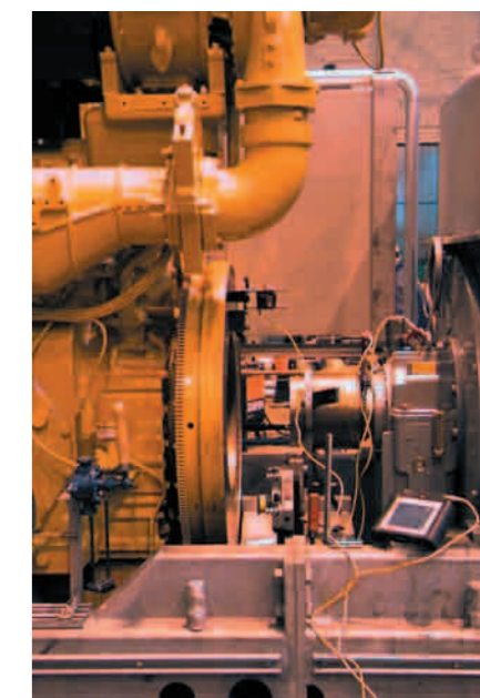
Alignment of engine with a Fixturlaser® laser-based alignment system.
