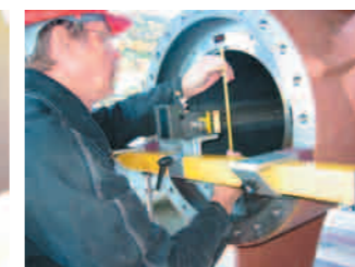
The stern tube is used as reference when measuring support bearings.
