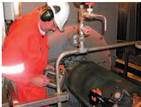
Machines move and grow from offline to running conditions. The Fixturlaser® laserbased alignment systems have the capability to measure and calculate with these specific deviation values.
