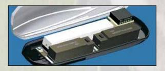
Rapid detection and identification of radioactive materials are made more likely with the use of Sodium lodide (Nal) detectors which provide improved sensitivity and nuclide identification capabilities than systems based upon plastic scintillators. The RS-700's sensitivity can be increased by readily adding up to three additional detectors and detection of Special Nuclear Materials (SNM) can be enhanced with the addition of the optional neutron detector.
