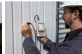
Measurement of a paint coating on steel
